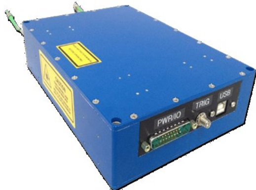
Fig. 2. Packaged hybrid HDFA/TDFA ( 200 \times 150 \times 43 \text{ mm}^3 ).
