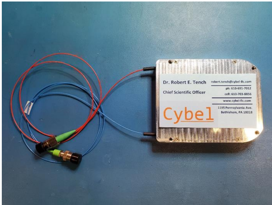
Figure 1. Miniature high wavelength HDFA with dimensions of 97 \times 78 \times 15 mm 3 .
