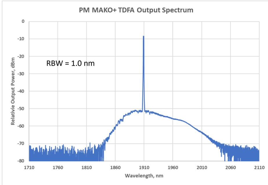
Figure 7. Measured Output Spectrum of the PM MAKO+ TDFA at 5.6 A Drive Current.
