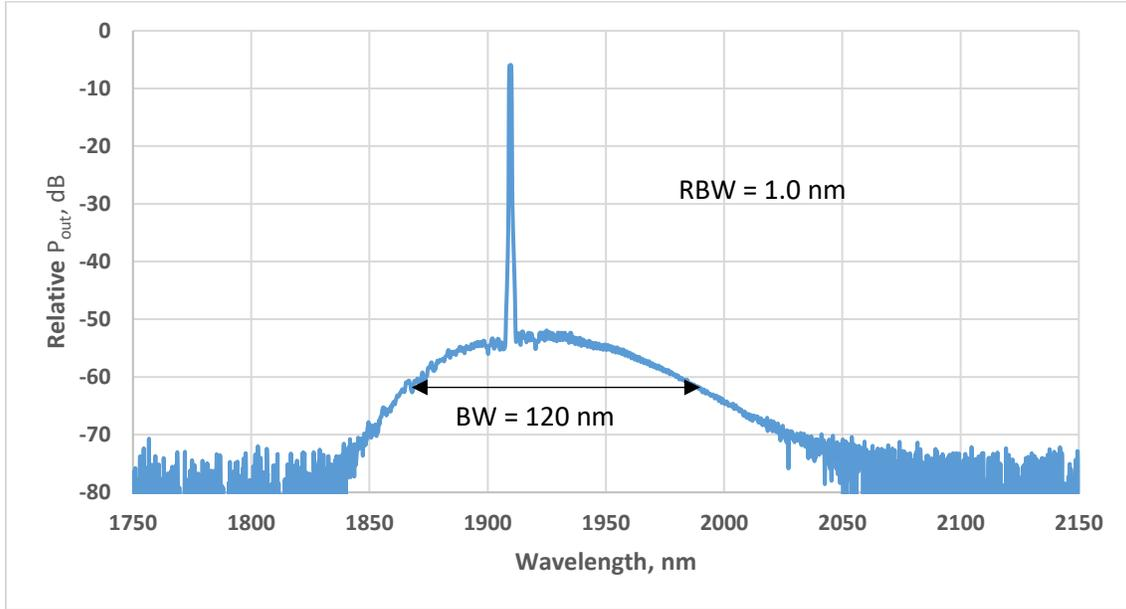
Figure 3. Single Stage Co-pumped PM TDFA Output Spectrum with  $P_s = 0$  dBm at 1909 nm for brassboard co-pumped amplifier.
