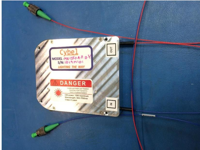
Figure 5. Miniature Packaged PM MAKO+ TDFA with Dimensions of  $97 \times 78 \times 15 \text{ mm}^3$  and Mass of 180 gm
