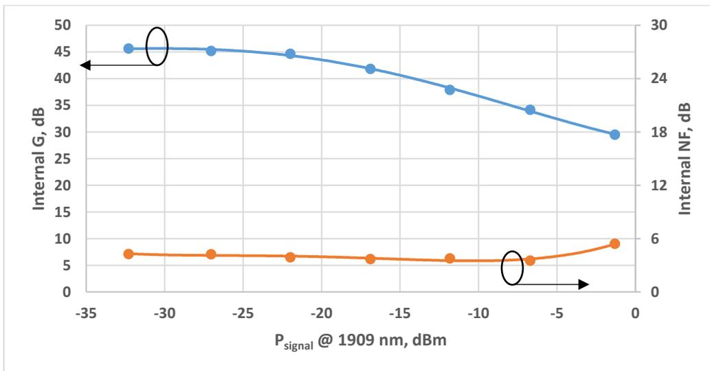
Figure 4. Internal G and NF for the Co-pumped Brassboard PM TDFA
