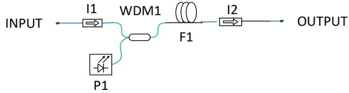
Figure 1. Optical design of co-pumped single clad polarization maintaining TDFA
