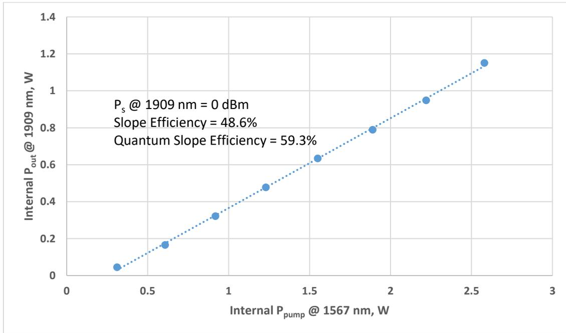
Figure 2. Internal  $P_{out}$  vs. Internal  $P_{P1}$  with  $P_s = 0$  dBm for brassboard co-pumped amplifier
