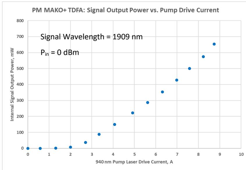
Figure 6. L-I Data for the Miniature MAKO+ PM TDFA
