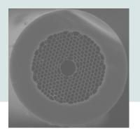
Optical signal in a hollow core photonic bandgap fibre is guided in an air core surrounded by a high air filling factor PBG microstructured region (>90%). Added to the low bend sensitivity due to the core high NA, this confers to this fibre design significantly reduced material nonlinearities since more than 95% of optical power is propagating in air. In addition air/undoped silica provides excellent temperature immunity critical for high performance fibre sensing and metrology applications.
