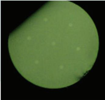
These Ge-doped silica multicore fibres integrates 7 photosensitive cores (6 hexagon-arranged cores around a center core) which make them particularly suited for Bragg grating inscription and sensing application (Shape, Strain, Temperature...) in the C-band. On-demand custom fiber design possible: core numbers, core location and composition.
