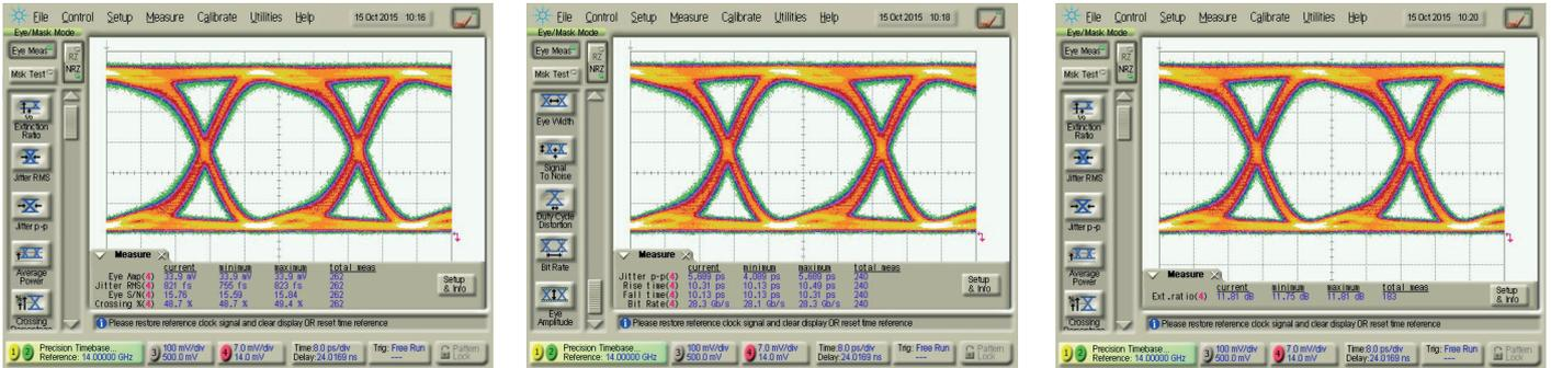
Eye Diagrams - 28 Gb/s - 1550 nm - From ModBox-1310nm-1550nm-28Gb/s-NRZ
