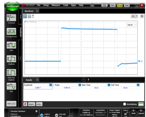
Output response: Pulse amplitude = 4.8 V pp , Rise time = 32 ps
