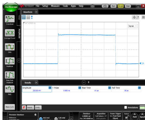
Input signal: Pulse amplitude = 0.25 V pp , Rise time = 32 ps
