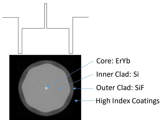
*All Glass Design : an extra layer of Fluorine doped Silica (SiF) is added between the silica clad and coating*
