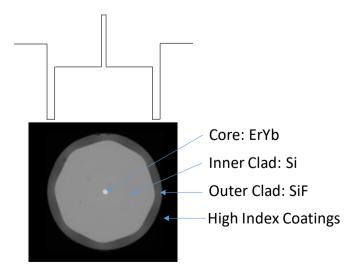
All Glass Design: an extra layer of Fluorine doped Silica (SiF) is added between the silica clad and coating
