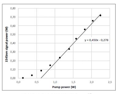
IXF-2CF-AG-EY-O-5-105-125-HTC in amplifier Background pump @ 976 nm; Pin = 10 dBm; 4.7 m
