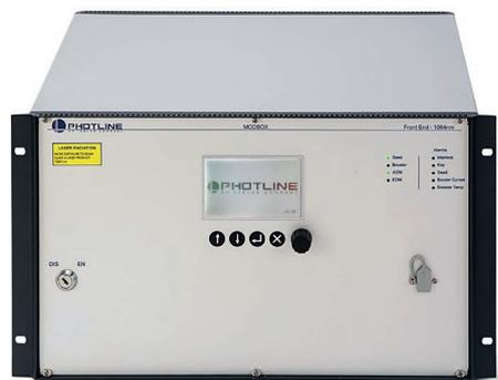
The Photline Modbox-Pulse-Shaper is an Optical Modulation Unit to generate short bespoke shaped pulses with high extinction ratio at 1030 nm, 1053 nm or 1064 nm. It allows dynamic extinction ratio from 35 dB to above 55 dB with user adjustable pulse duration, repetition rate and temporal pulse shape. One benefit of the Photline Modbox-Pulse-Shaper is to pre-compensate the pulse distortion that occurs in the amplifiers chains that operate in (a highly) saturated regime.
