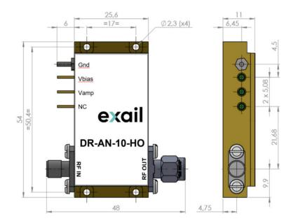
The heat-sinking of the module is necessary. It's user responsability to use an adequate heat-sink. Refer to page 5 for Exail
