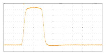
Pulse Width: 20 ns Output voltage: 8 Vpp
